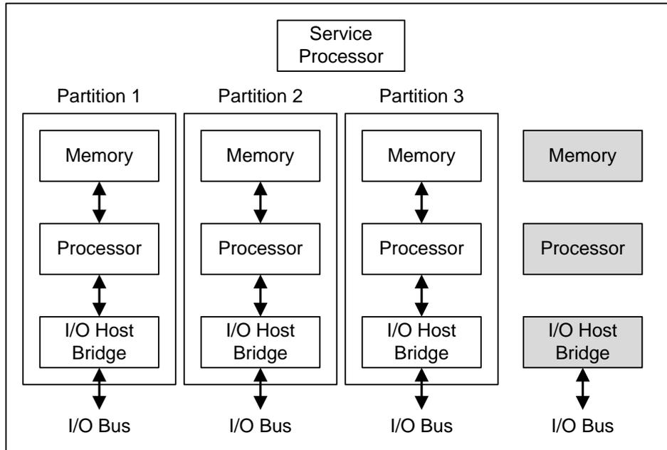
In this example each partition unit consists of a single hardware component (a processor, memory module, or I/O host bridge). However, today's hardware partitionable servers typically have multiple hardware components in each partition unit. This simplified example is used here for illustration purposes.
