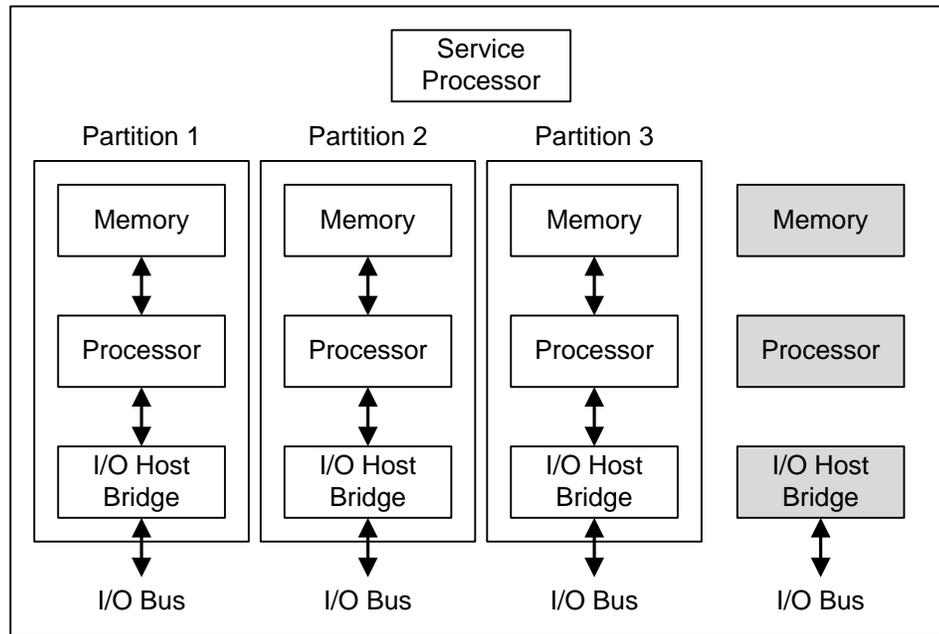
In this example, the server has a total of 12 partition units: 4 processors, 4 memory modules, and 4 I/O host bridges. One of each of these three types of partition units is assigned to one of three hardware partitions. The remaining partition units are available as spares that can be used to add hardware resources to one of the hardware partitions or to replace a failing partition unit in one of the hardware partitions.
